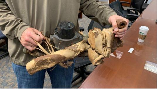
Paradise Irrigation District manager Kevin Phillips shows a sample of the town's water pipes, which were frequently woven between underground root systems that were likely burned during the fire.
